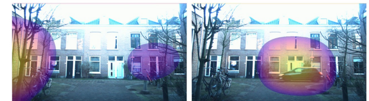
(c) sound localization with a vehicle-mounted microphone array detects the wall reflection of an approaching vehicle behind a corner before it appears
